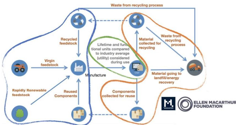
The measurement method of the Madaster CI has three different phases: the construction phase (blue), the use phase (green), and the end-of-life phase (orange). This enables users to compare products and buildings by comparing the various components and to easily assign circularity ambitions and objectives.
