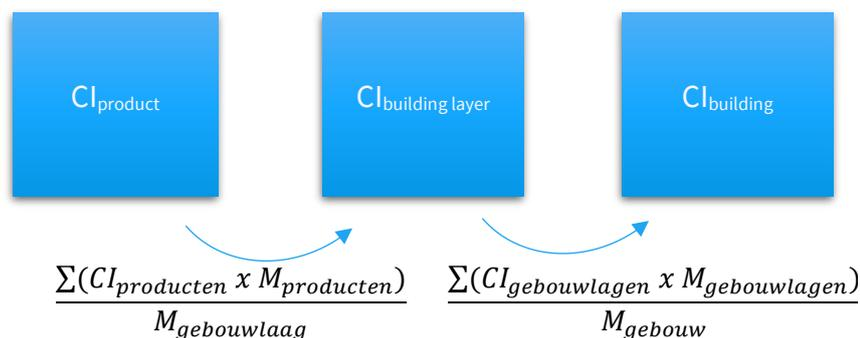
The Madaster CI measurement method consists of two levels:
